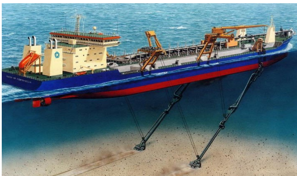
Figur 6.7. Illustration af Trailing Suction Hopper Dredger (TSHD).
