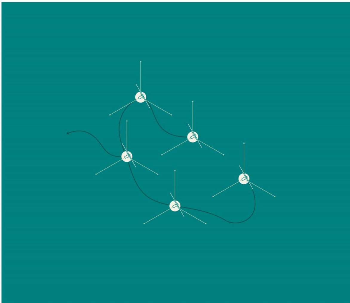
Figure 12. Top view showing how the turbines with associated anchorage lines are connected via the inter-array cables. Illustrator: Tobias Green.
