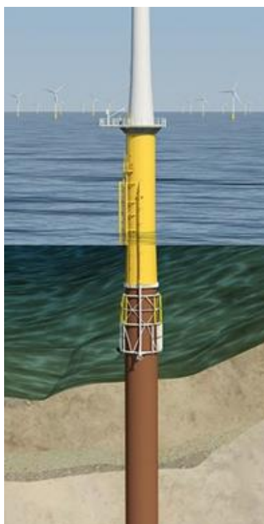
Figure 8. Monopile foundation. Illustration COWI
