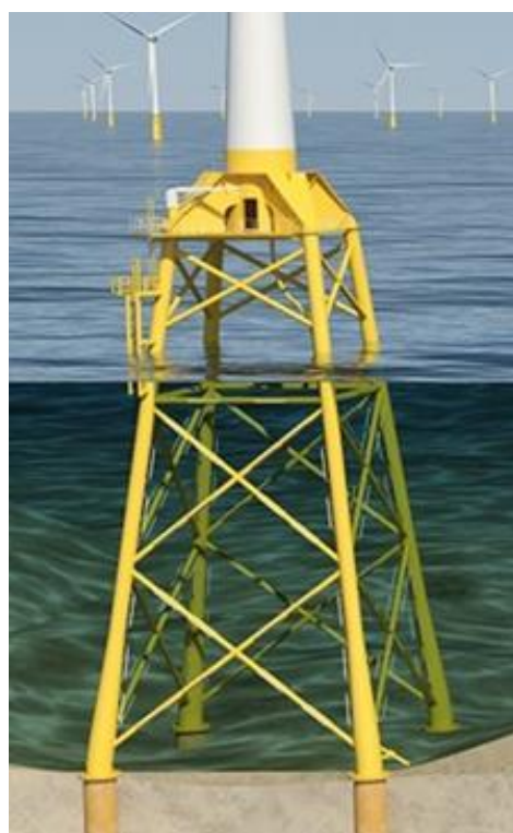
Figure 9. Jacket foundation Illustration COWI
