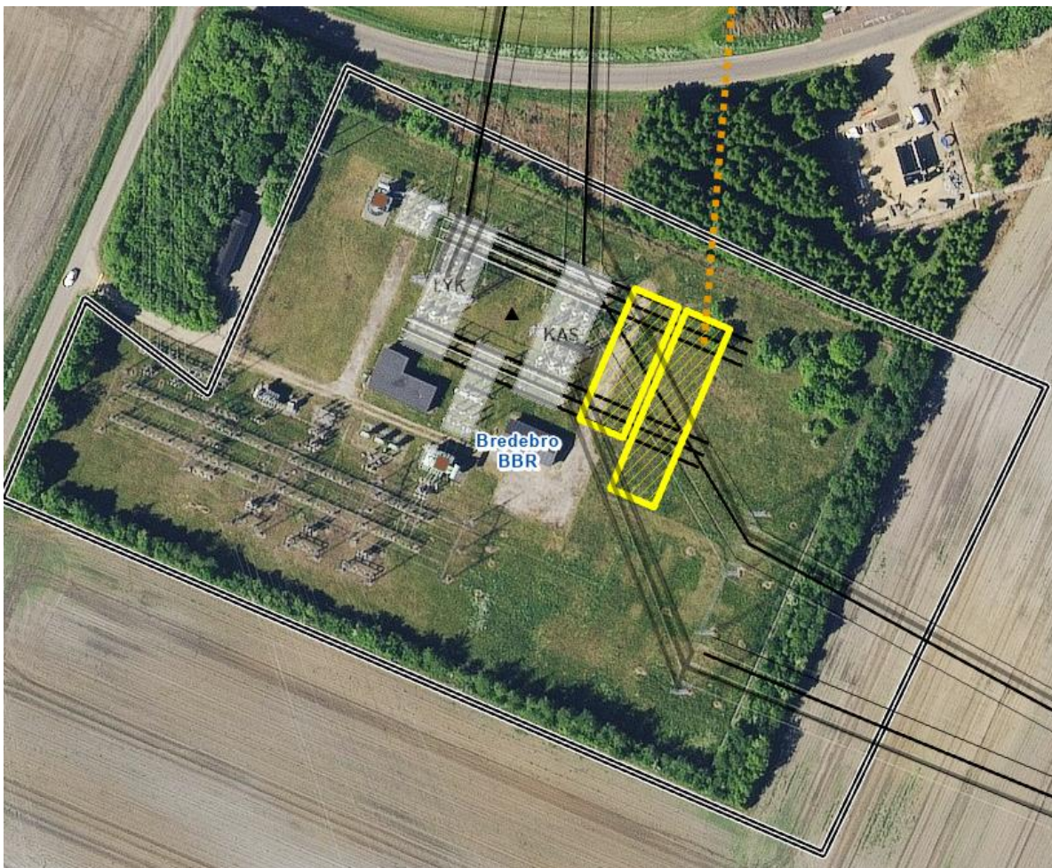
Figur 2- Layout of 150 kV station Bredebro, gul indikerer de to nye felter der skal etableres
