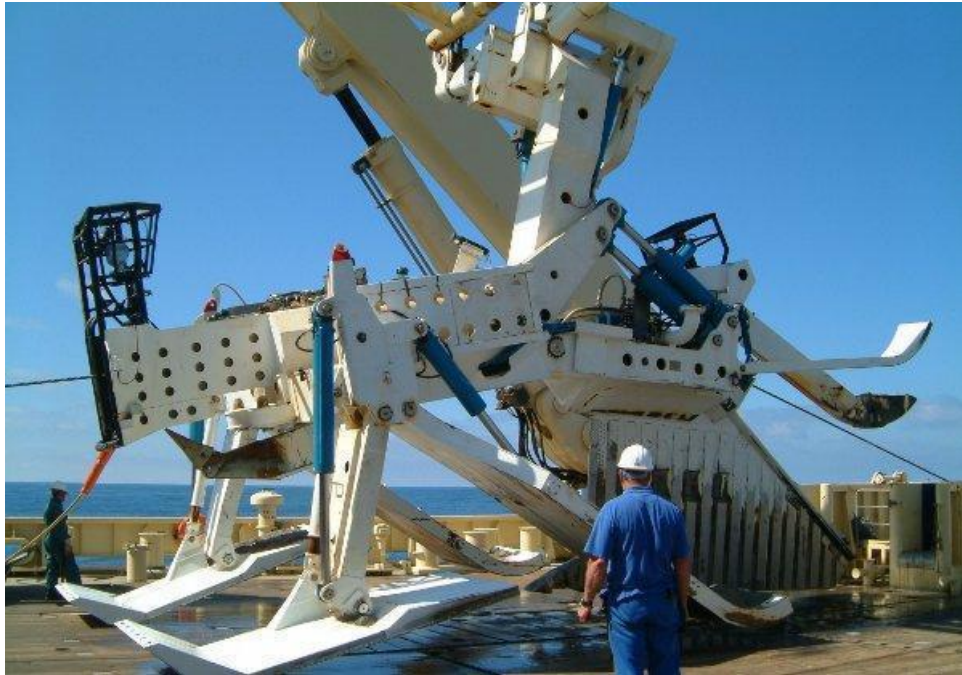
Figur 27: Udsigt over Pharos Offshore Group Ltd's plov til installation af undersøiske kabler (Kilde: http://www.4allports.com/images/equipment/42/42.jpg )
