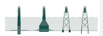
Figure 3. Principle sketch of bottom-fixed foundation alternatives. (From left: monopile foundations, gravity foundations, jacket foundations with suction buckets and jacket foundations with pin-piles). Source: Landinfra.
