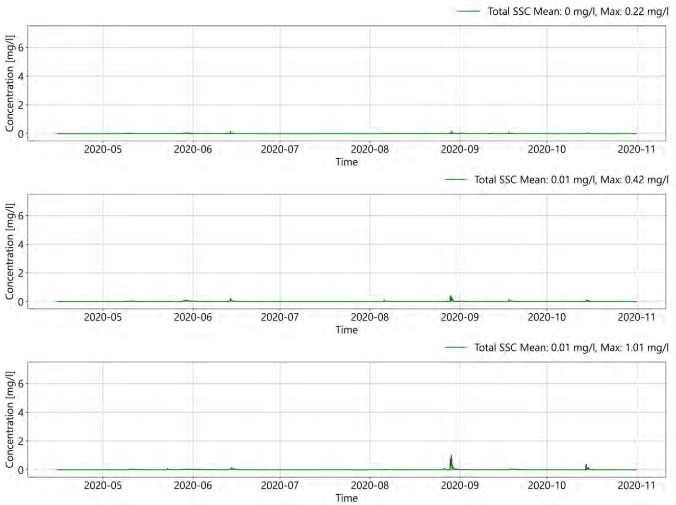
Point 2 : Timeseries of concentration for: the: top 2 meters (top figure), depth-averaged over the entire water column (middle figure) and bottom 2 meters (bottom figure). Geographical location in Figure 6.1.
