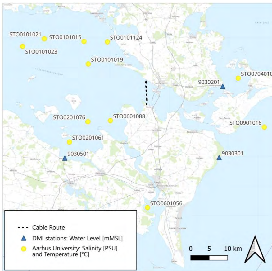
Figure 4.2: Overview of stations where data on water level, salinity and temperature are extracted from.
